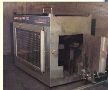
Flame test equipment (Interior part)
