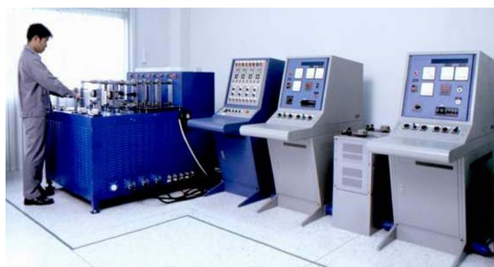
Apparatus for making and breaking capacity and normal operation test
