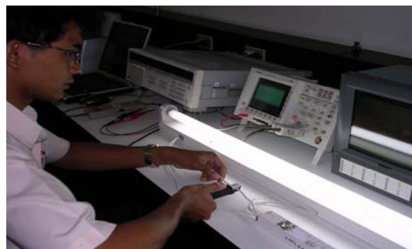
Electronic ballast testing
