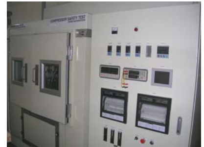
Running overload test of motor-compressor (Annex AA IEC 60335-2-34)
